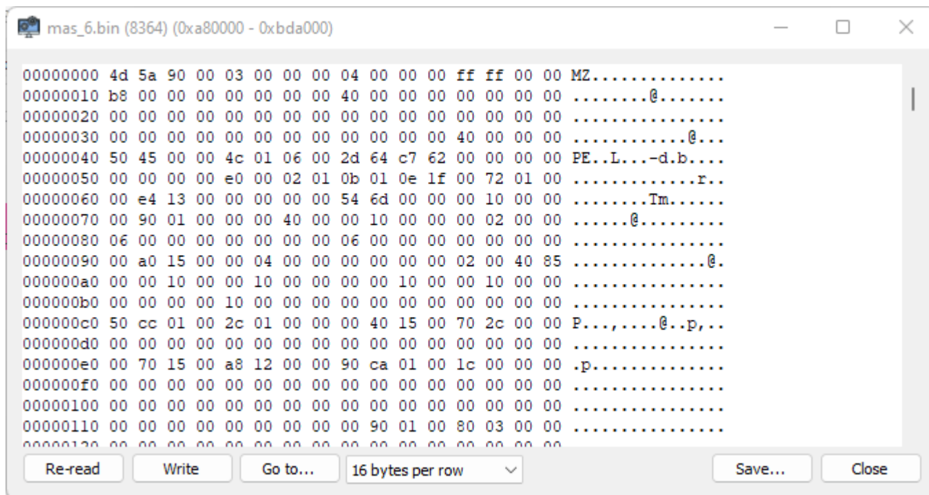
[Figure 32] System Informer (Process Hacker): visualizing the PE file in the second region
